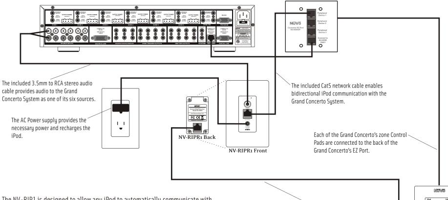
The NV-RIP1 is designed to allow any iPod to automatically communicate with the new Grand Concerto Audio Distribution System. The included dock can be located in any zone of the house and requires just a single Cat5 connection from the dock to the NV-RJ45P component located in the wall. Additionally, a single Cat5 run from the back of the RJ45P to the back of the NV-RIPR1 iPod receiver component located with the Grand Concerto main amplifier transmits power, audio signal and metadata.
